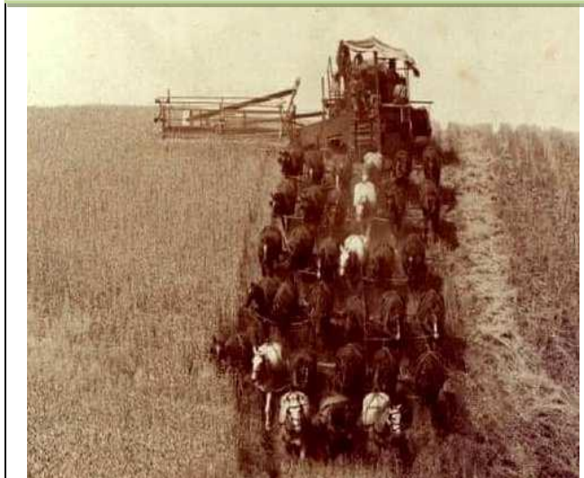
This is how they did it in the good old days! A 33 horse wheat harvester from the 1900's.
